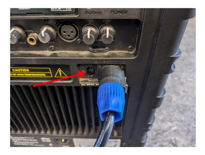
To connect the cable: plug it in and turn it clockwise until it clicks into place:
