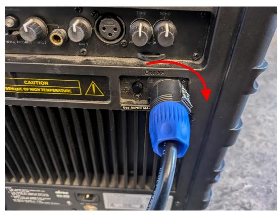
To release the cable again, you have to pull the lock backwards and turn the plug to the left:
